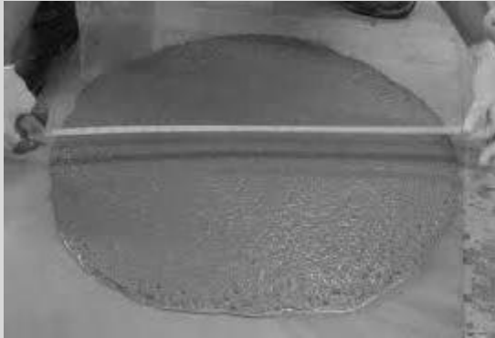
Figure 14: Measuring the spread of self consolidating concrete (Credit: NRMCA)
